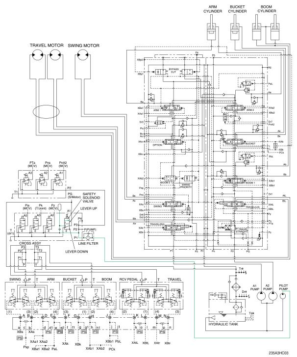
When the lever of the safety solenoid valve is moved upward, oil flows into the remote control valve through the line filter, safety solenoid valve and cross assy.
